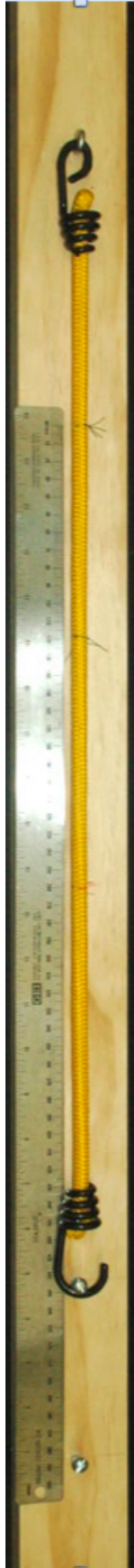
Figure 1. Example of the apparatus for Activity 1. Black threads are sewn around the cord on the left side. A red thread is sewn about 2/3 of the way to the right. Cronin, 2012.
